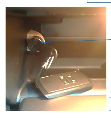
« Keyfob » allowing to detect the presence of the keys.
